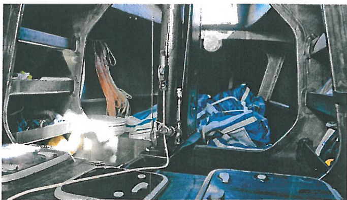
Home sweet home, with the keelbox in the foreground. The custom-made header tank for the canting keel's hydraulic fluid is installed with the pumps in the keel compartment, which reduces the amount of piping
