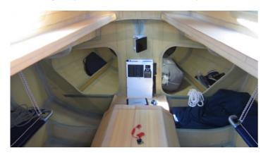
Down below the finish is bare glass with the engine box in the middle of the saloon and with the galley and nav station on the main bulkhead. There is a pipecot on either side of the main 'saloon' area and a plumbed in head mounted on the forward side of the main bulkhead.
